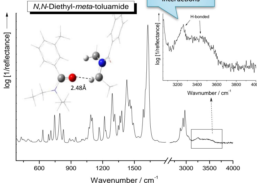
Bands related to symmetric and asymmetric stretching vibrations of OH groups are localized in frequency range:
