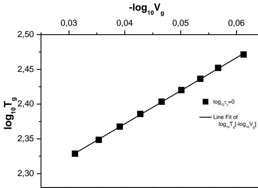
At  $T=T_g \Rightarrow T_g^{-1} V_g^{-\gamma} = \text{const.}$
